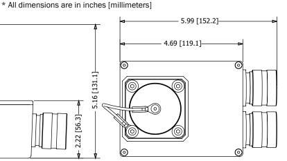
DC Receptacle Protective Cap Tesla™ NATO DC Receptacle Compression Grommets
