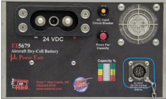
Figure 3.12.1 AC Input Connector (outlined in blue)
