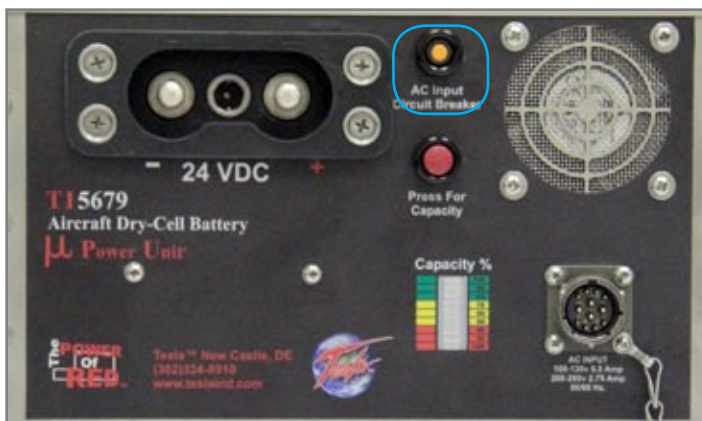
Figure 3.13.1 AC Input Circuit Breaker location (outlined in blue)
