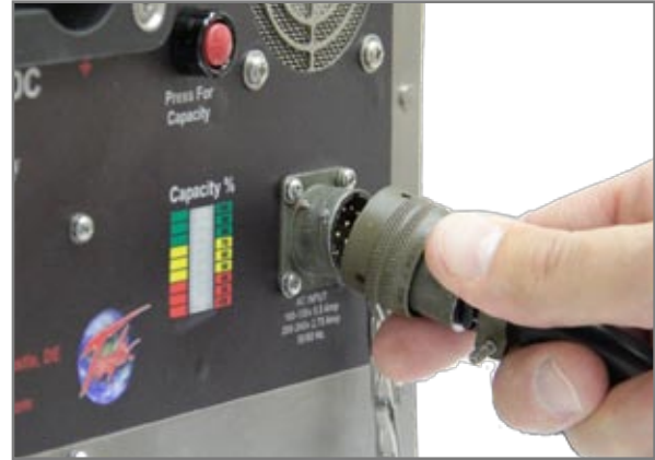
Figure 3.12.2 Attaching AC Line Cord
