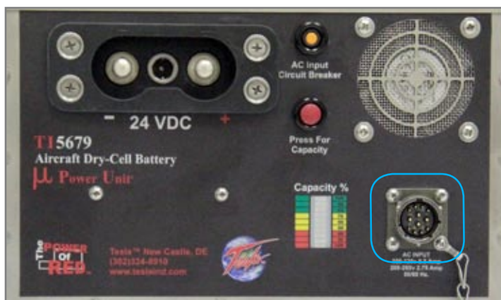
Figure 3.14.1 AC Input (outlined in blue)
