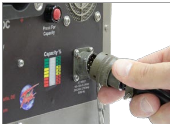
Figure 3.14.2 Attaching AC Input Line Cord
