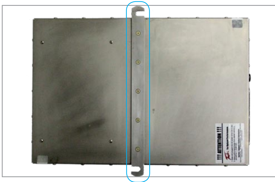
Figure 3.8.1 – Battery Lock-down (outlined in blue)
