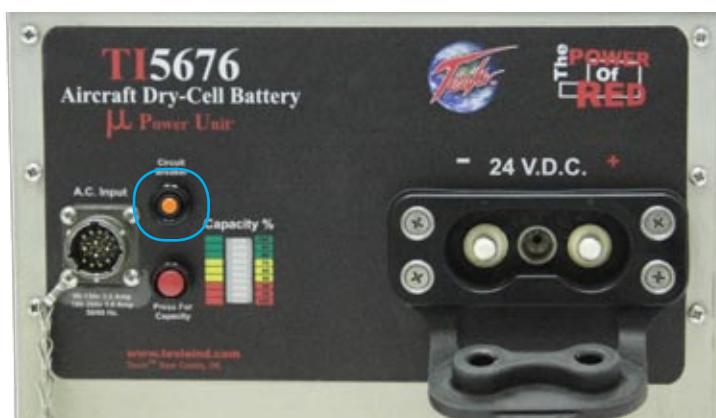
Figure 3.9.1 AC Input Circuit Breaker location (outlined in blue)
