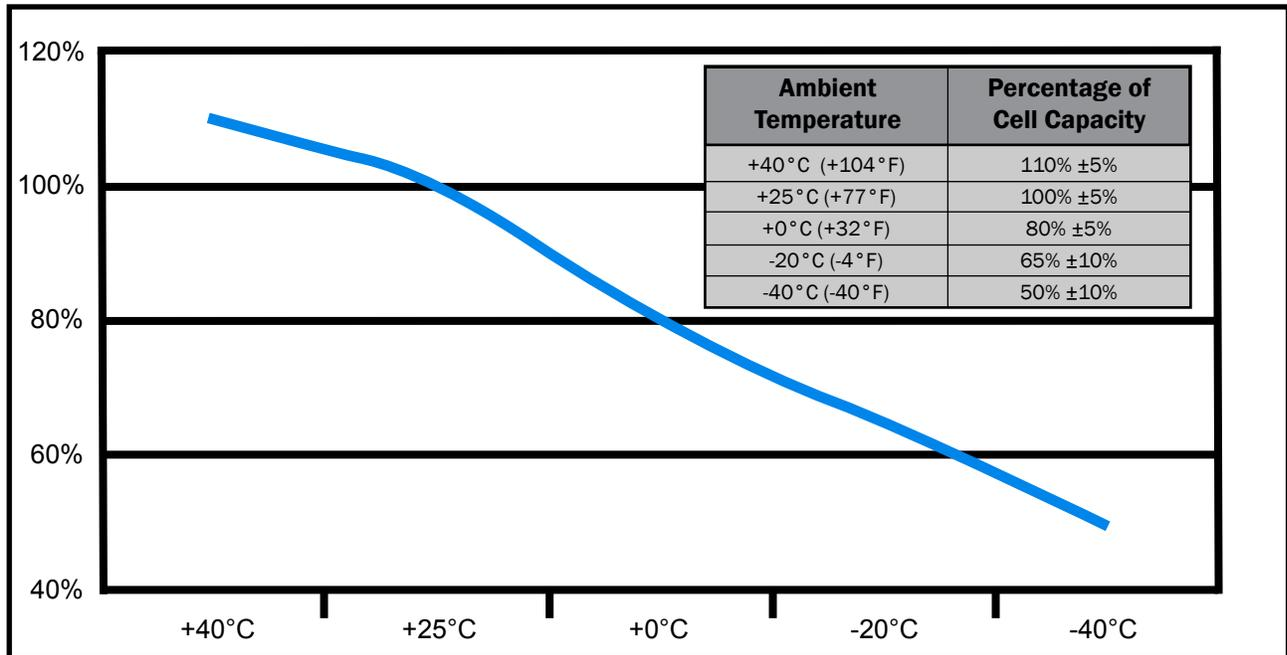
Figure 4.7.1 – Cell storage capacity versus ambient temperature
