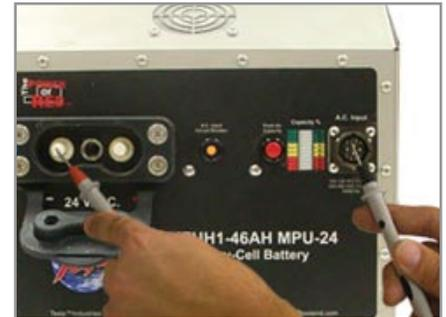
**3.** Move the positive probe to the dc negative post on the DC Output Connector.
