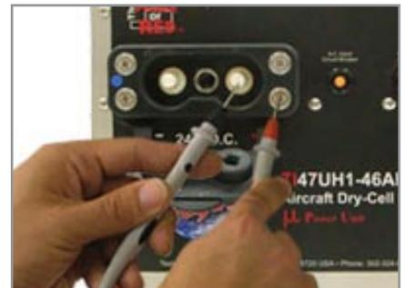
**6.** Move the negative probe to the dc positive post on the DC Output Connector.
