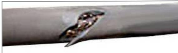
Figure 6.1.1 – Damaged cable
