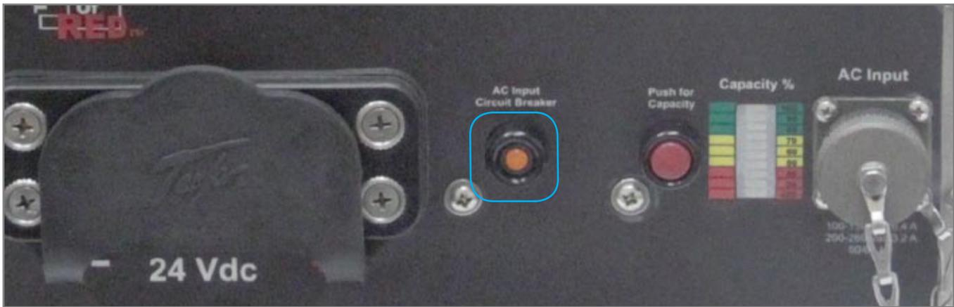
Figure 3.2.1 AC Input Circuit Breaker location (outlined in blue)
