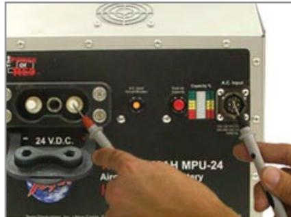
**2.** Move the positive probe to the dc positive post on the DC Output Connector.
