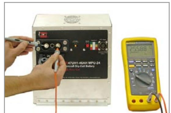
Figure 4.9.3 – Testing DC Receptacle
