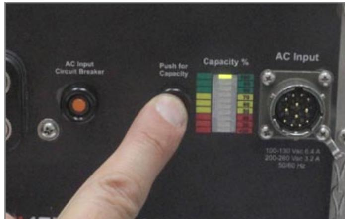
Figure 3.4.1 Pushing to Test
