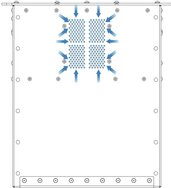
Figure 2.6.1 Back of Unit: Rear Inlet
