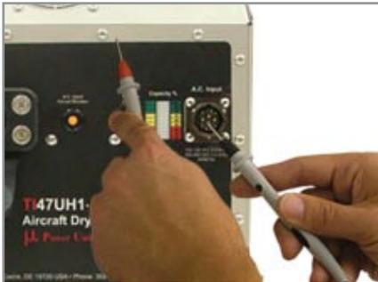
**1.** Place the negative probe on the ac ground probe ( J or L) and the positive probe on an exposed part of the metal case.
