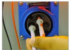
**1.** Place the negative probe on the receptacle's left ground insert and the positive probe on top side phase 1 insert.
