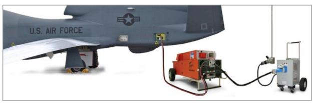
Figure 6.6.1 Connecting DC cable to aircraft and starting engine
