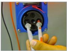
**2.** Move the positive probe to the right side phase 2 positive insert.
