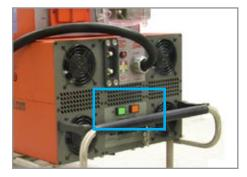
Figure 6.5.1 DC "ON/OFF" buttons location.
