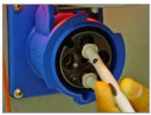
**2.** Move the positive probe to the lower phase 3 positive post.
