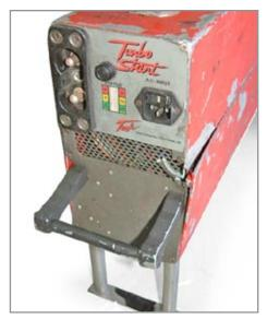
Figure 8.2.2 – Damaged Unit Misaligned Case with Bent Faceplate
