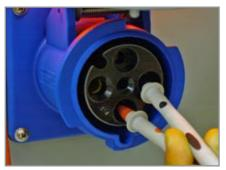
**3.** Move the negative probe to the right side phase 2 probe and the positive probe to lower phase 3 probe.
