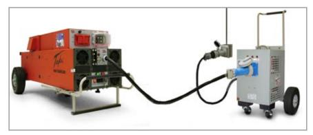
Figure 6.4.1 Transformer connected to GPU
