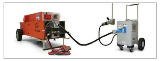
Figure 6.5.3 DC cable plugged into GPU.
