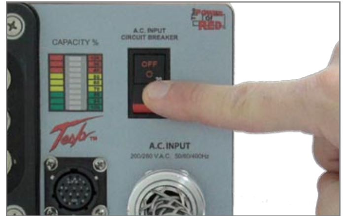
Figure 3.9.1 - Turning On AC Input Circuit Breaker
