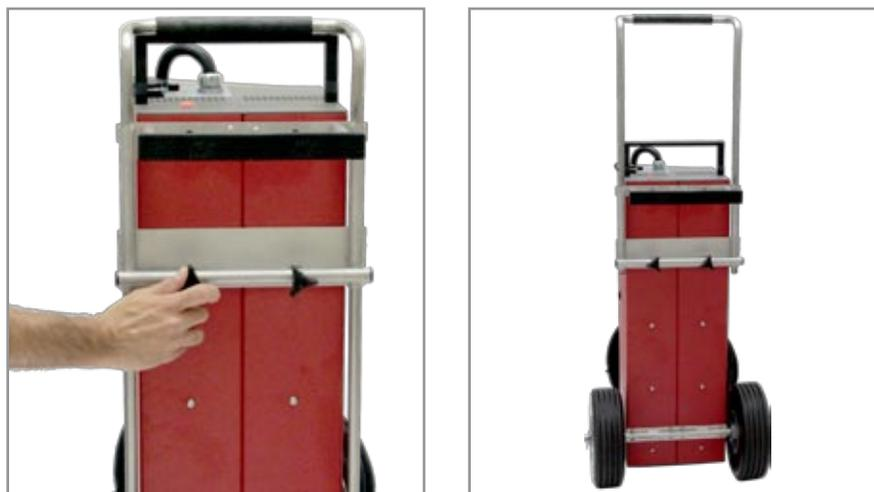
Figure 3.10.1 Releasing Telescopic Handle
