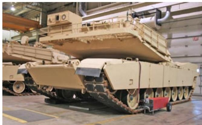
Figure 3.11.3 Starting vehicle with TI5200 GPU-24
