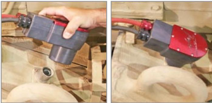
Figure 3.11.2 Attaching NATO DC Power Cable to vehicle
