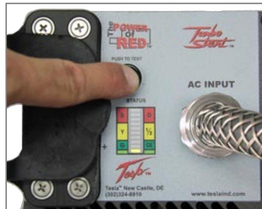
Figure 2.8.1 - Pushing to Test
