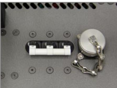
Figure 3.16.5 Circuit Breaker OFF
