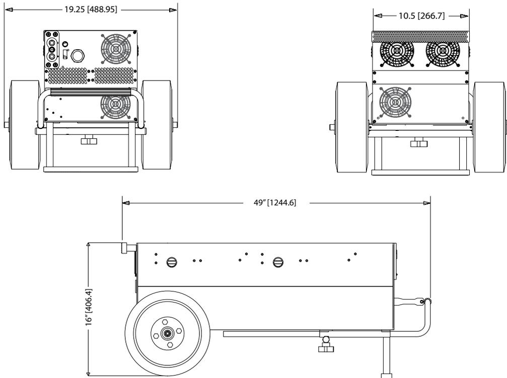
Figure 2.5.1 – TI5200 GPU-24 physical dimensions
