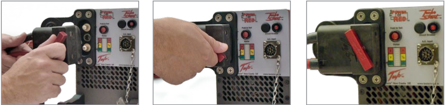
Figure 3.11.1 Attaching DC Power Cable to TI500 GPU-24
