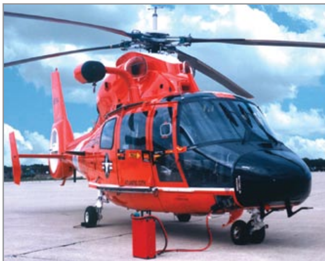
Figure 3.11.1 Starting aircraft with TI500 GPU-24
