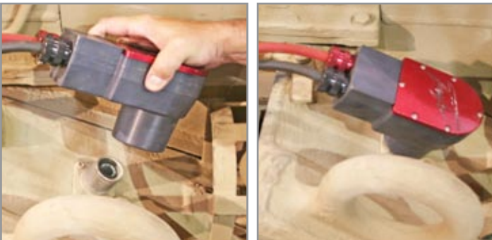
Figure 3.11.2 Attaching NATO DC Power Cable to vehicle
