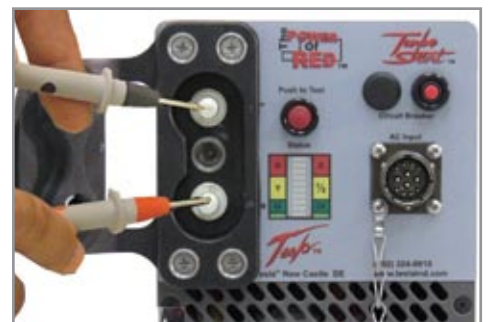
Figure 3.8.3 – Testing DC Receptacle
