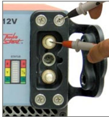
3.8.4 - DC Output Connector Positive Pin
