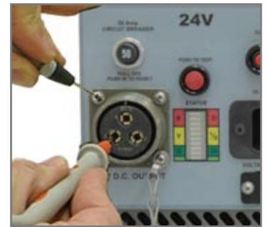
3.8.7 - DC Output Connector Positive Pin
