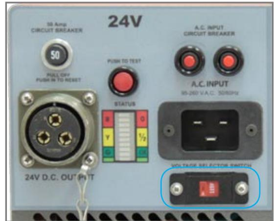
Figure 2.13.1 Input Voltage Selector Switch (outlined in blue)
