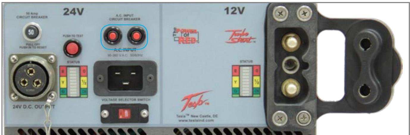
Figure 2.8.1 - AC Input Circuit Breaker (outlined in blue)
