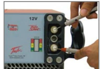
3.8.8 - Measuring Voltage on DC Output Connector
