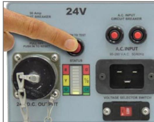
Figure 2.14.2 - Pushing to Test
