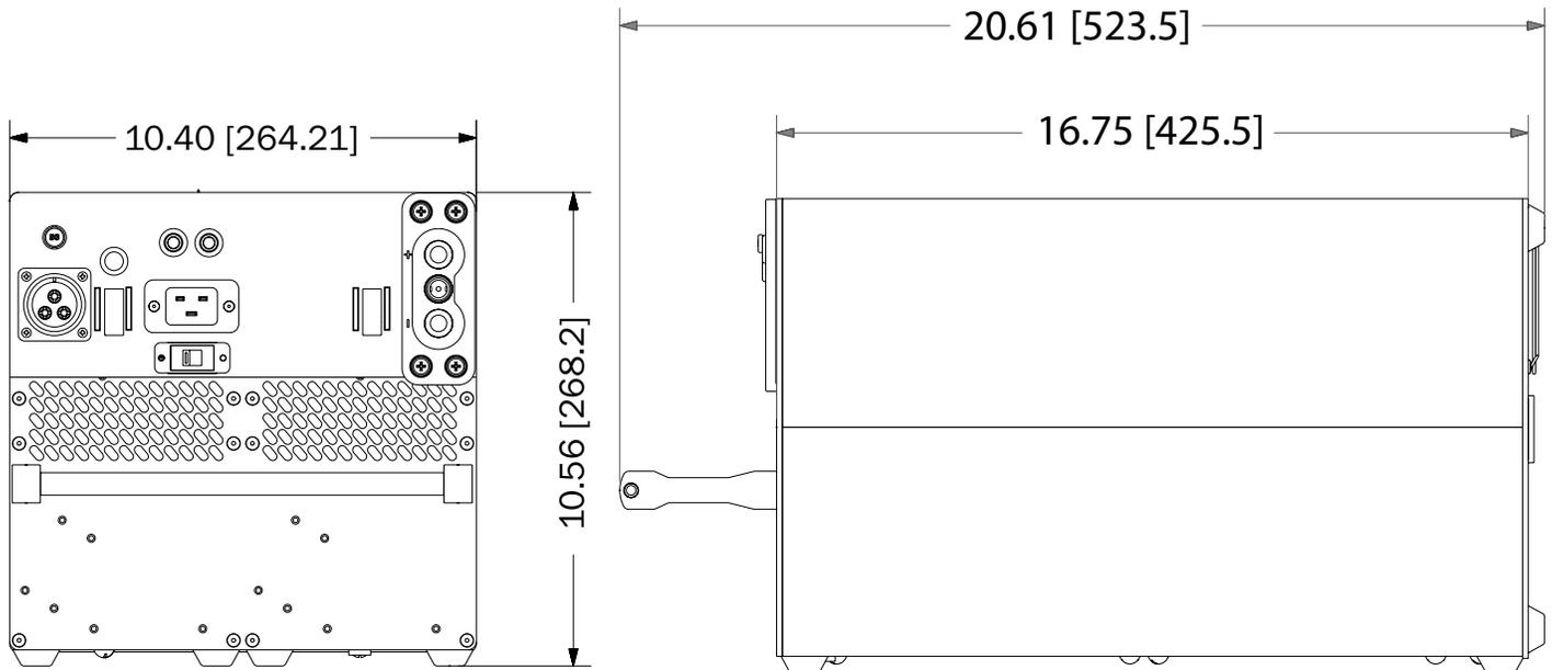
Figure 2.5.1 – TI1550 12-24-UAV GPU physical dimensions
