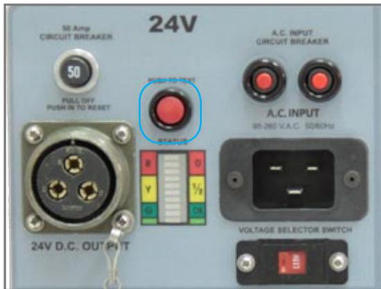
Figure 2.14.1 - “Push to Test” button location (outlined in blue)
