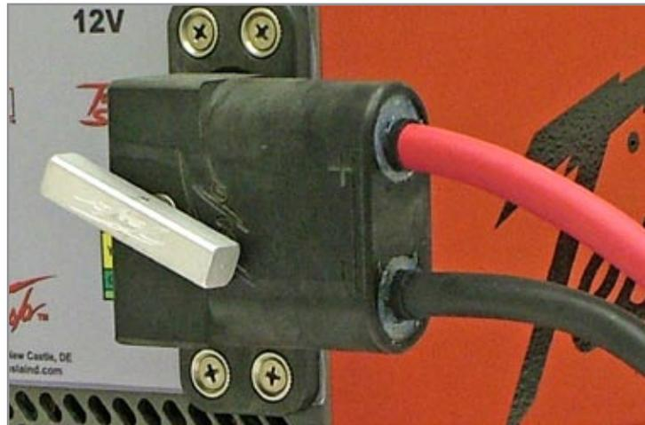
Figure 3.11.1 Attaching DC Power Cable to GPU
