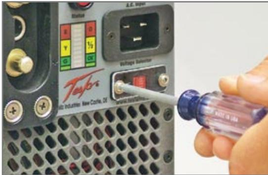
Figure 2.13.2 - Unscrew Protective Cover
