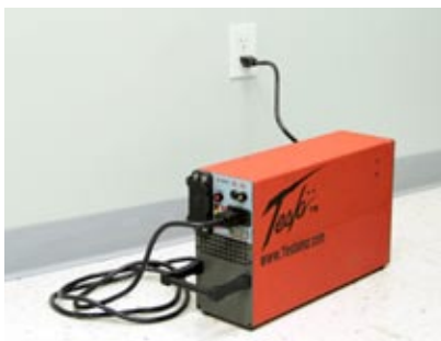
Figure 4.3.1 Connecting TI1530 GPU-12 to AC Power Supply
