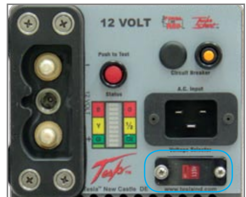
Figure 1.3.4 – TI1530 GPU-12 Input Voltage Selector Switch
