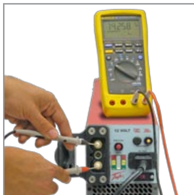
Figure 3.8.2 – Testing DC Receptacle
