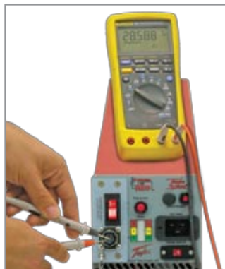
Figure 3.7.2 – Testing DC Receptacle
