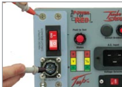
2. Place the positive probe to the fastener screw on the dc post. Move the negative probe to the dc negative post (A). Multimeter should read 0 Volts.
