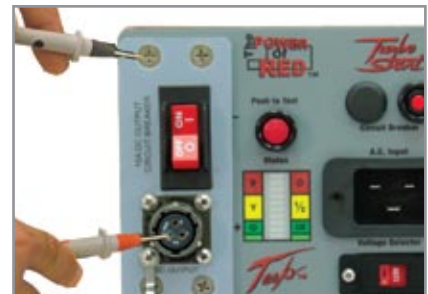
3. Place the negative probe to the fastener screw on the dc plate. Move the positive probe to the dc positive post (C). Multimeter should read 0 Volts.
