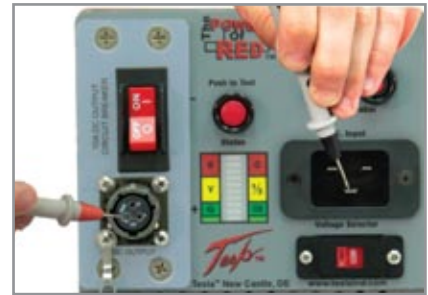
2. Place the negative probe on the ac ground post and the positive probe to the dc positive post (C). Multimeter should read greater than 10 MΩ.
