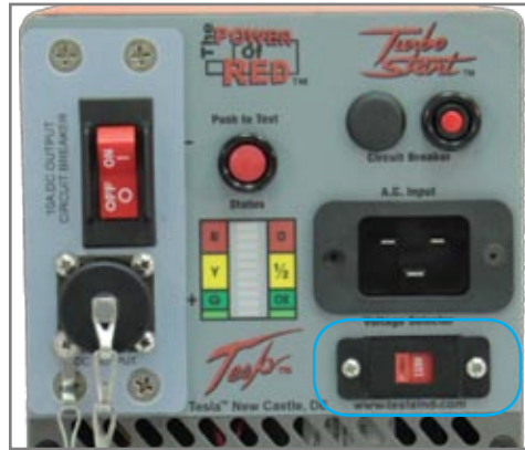
Figure 2.10.1 Input Voltage Selector Switch (outlined in blue)
