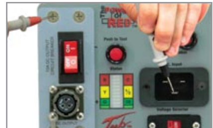
6. Move the positive probe to the fastener screw on the dc plate. Multimeter should read less than 1Ω.
