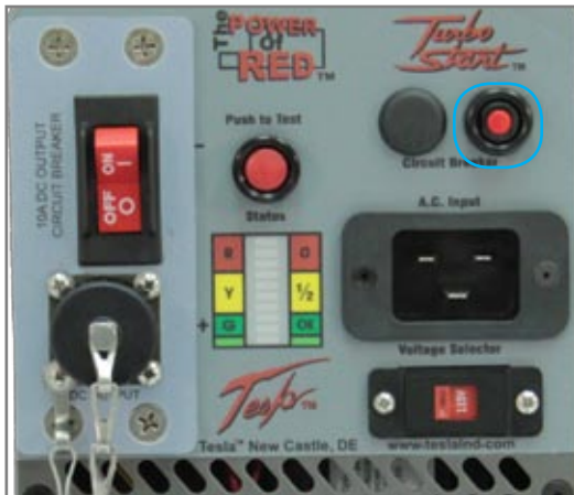
Figure 2.8.1 - AC Input Circuit Breaker (outlined in blue)
