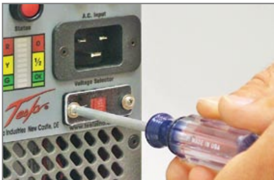
Figure 2.10.2 - Unscrew Protective Cover
