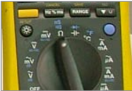
1. Set multimeter to Ohms.
