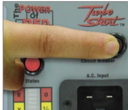
Figure 2.8.2 - Pressing Circuit Breaker
