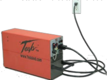
Figure 3.10.1 Connecting TI1000 GPU-24 UAV to ac power supply
