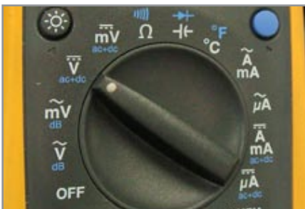
1. Set multimeter to Volts.
