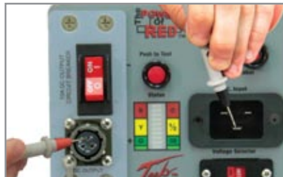
5. Move the positive probe to the pin (B) on the dc receptacle. Multimeter should read less than 1Ω.
