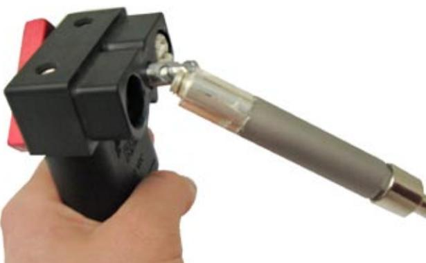
**Step 2:** Next, insert the tool into the contact and turn counterclockwise using the wrench.
