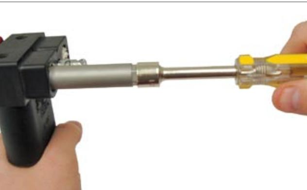
**Step 3 & 4:** To install a new contact, use the same tool and screw the contact in clockwise using a 3/8" torque wrench. Be sure to fully insert the tool or the fins may break.
