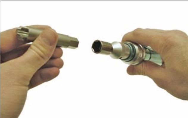
**Step 1:** To remove either contact, insert the hex end of the DC Contact Insertion/Extraction Tool into a 1/2 inch socket wrench. Do not use a torque wrench.
